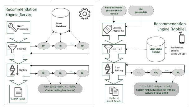
Figure 1: Design of the recommendation engine: (a) server-side engine with fully evaluated query, (b) client-side engine with partly re-evaluated query utilising local cache.
